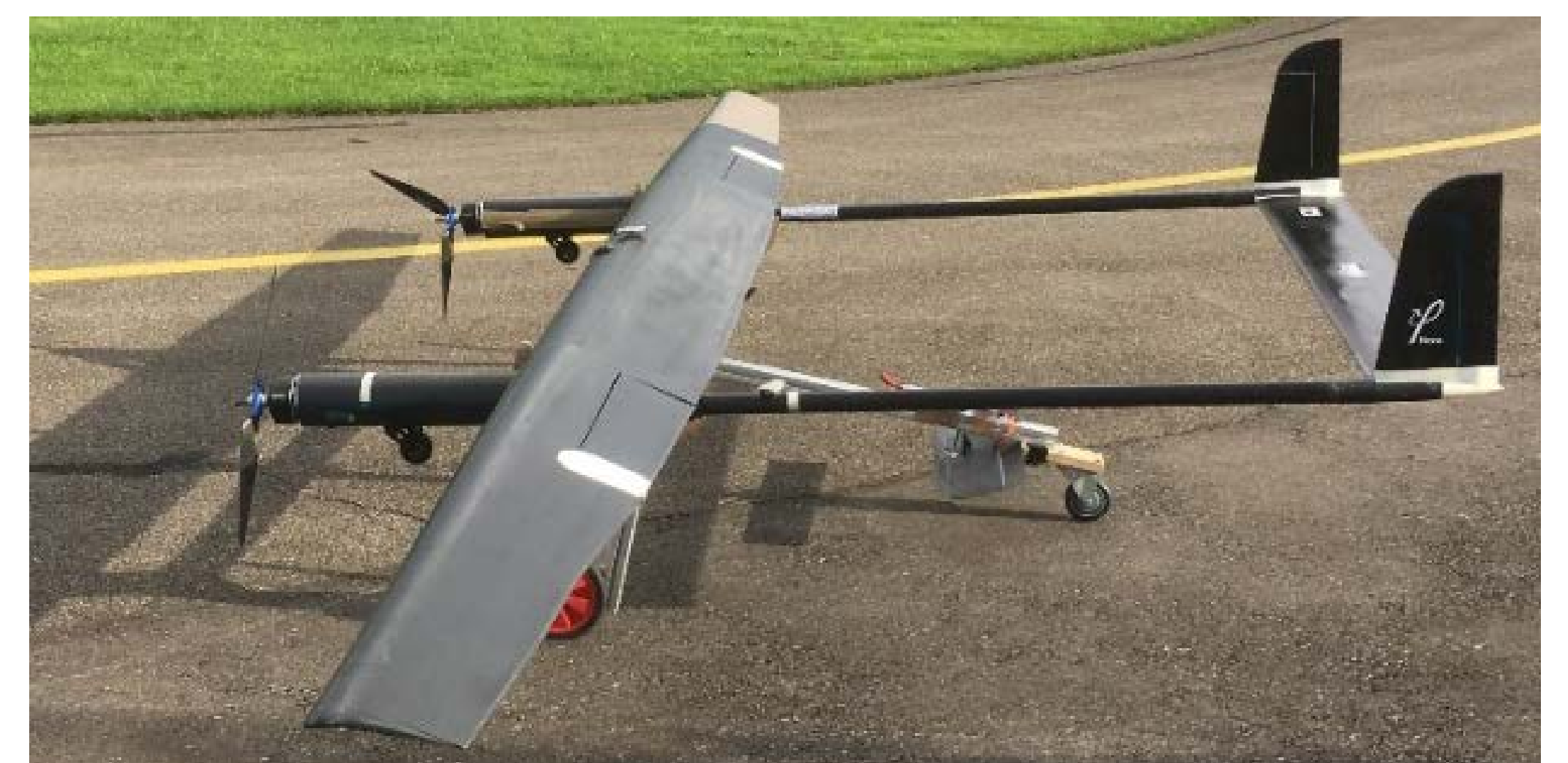
Morphing wing assembled for flight test
