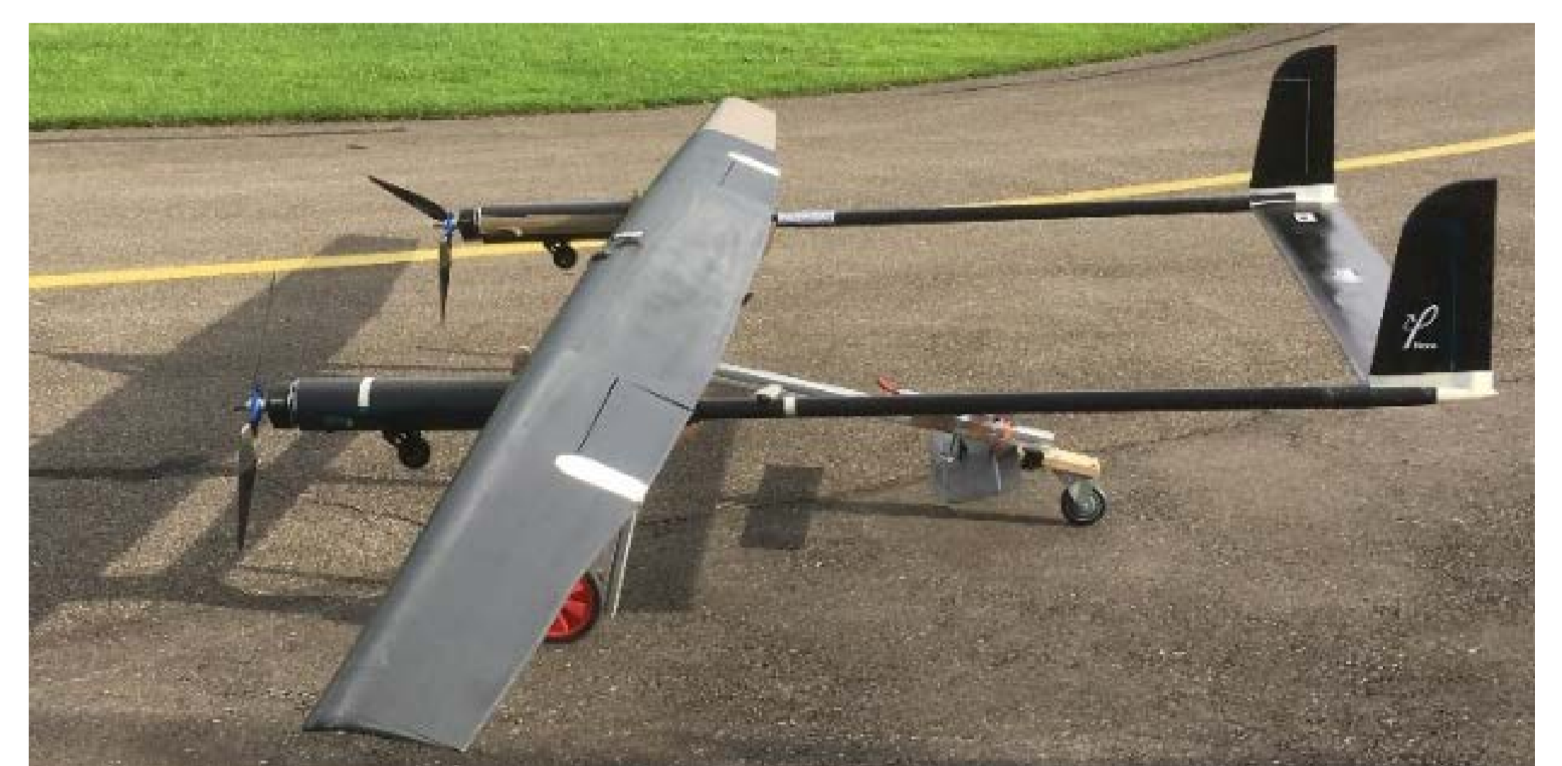
Morphing wing assembled for flight test
